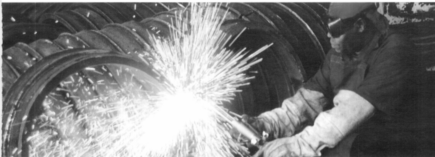
Metal cutting at Kenya Railways Central Workshop, using high purity Oxygen and Acetylene products from BOC Kenya Ltd.
